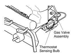
Figure 31 - Location of Gas Valve Assembly and Thermostat Sensing Bulb
